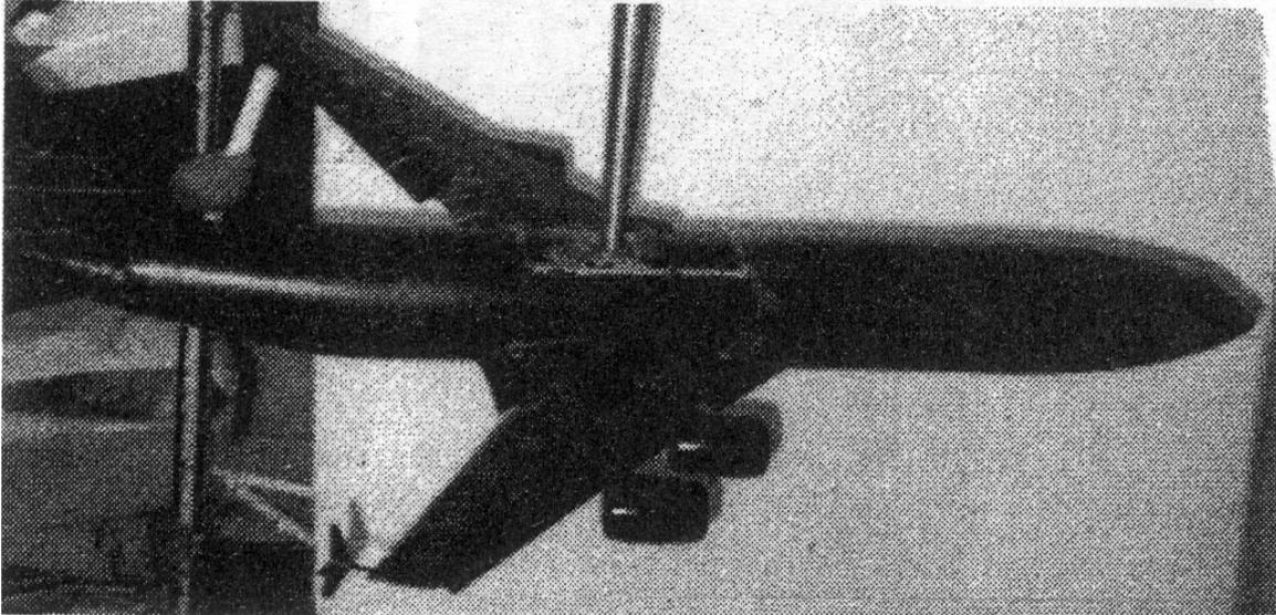
**Figure 3: Model of an aeroplane in the wind tunnel.**
